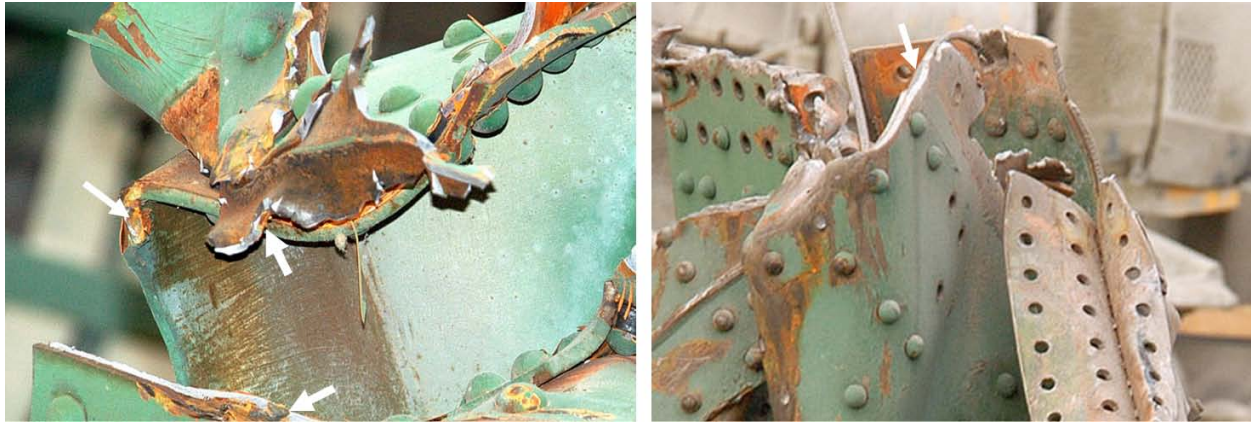
Fig. 11 Fractographies of wrecked gusset plates of I-35W bridge; these photos were made at the day after the collapse (downloaded from www.dot.state.mn.us/i35wbridge/photos/ground/aug2/ at 3/5/08). The rusted old surface parts surrounded by fresh fractured surfaces, as pointed by the white arrows, look like fatigue cracks. Some of them are in welded joints.
